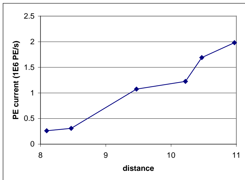
FIG. 48. PE rate vs. distance between lens and sample for Si wafer at 230 nm.
